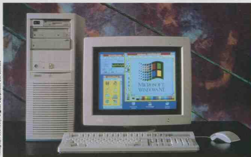
The DEC Alpha AXP isn't strictly speaking a PC, but it can run Windows NT and other Windows applications. It uses a very fast 66MHz RISC processor, but is decidedly expensive
